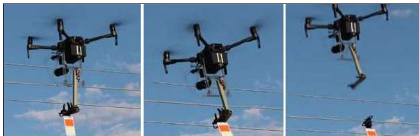
Drones provide a cost-effective and safe alternative for attaching line markers without risking human safety, revolutionizing traditional methods
