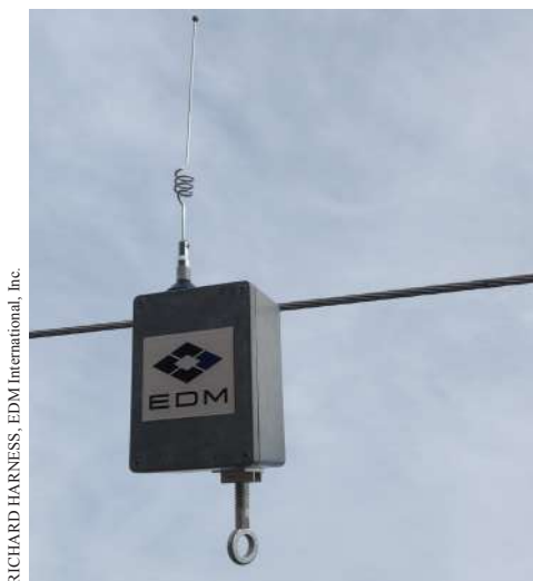
(Left): Utilizing advanced Bird Strike Indicators (BSI) is crucial for monitoring and mitigating potential collisions, providing valuable insights into bird behaviour around critical areas to enhance avian safety in proximity to power lines (Right): Smart vision cameras installed on a transmission pole capture passerines crossing a transmission line, offering direct monitoring for collision mortality on power lines
