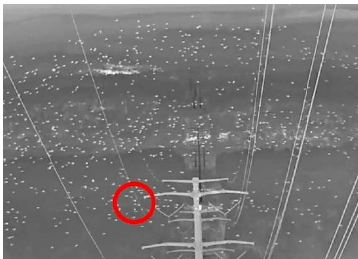
(Left): Utilizing advanced Bird Strike Indicators (BSI) is crucial for monitoring and mitigating potential collisions, providing valuable insights into bird behaviour around critical areas to enhance avian safety in proximity to power lines (Right): Smart vision cameras installed on a transmission pole capture passerines crossing a transmission line, offering direct monitoring for collision mortality on power lines
