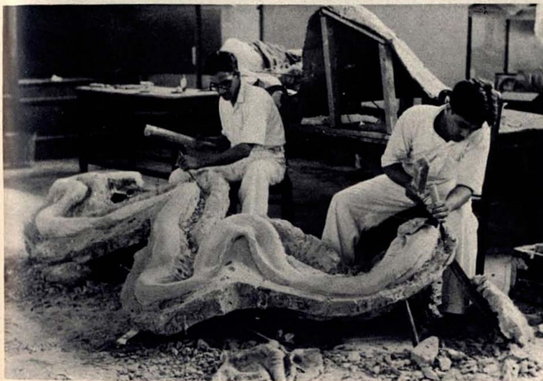
Chipping the mould off the cast
